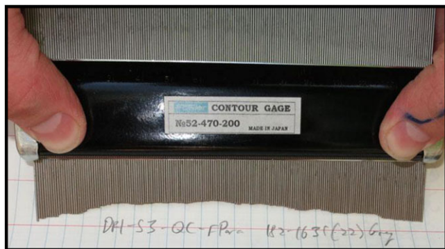
Figure 4. Contour gage photographed after being pressed perpendicularly against the bedrock surface. Photographs were processed using image analysis to determine surface roughness, calculated as the standard deviation of pin heights. [Colour figure can be viewed at wileyonlinelibrary.com ]
