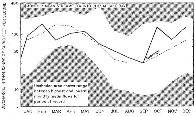
Figure 2. Monthly mean streamflow into Chesapeake Bay during 1990 (solid line) compared with average monthly mean flow for the thirty year period from 1960 through 1990 (dashed line).
