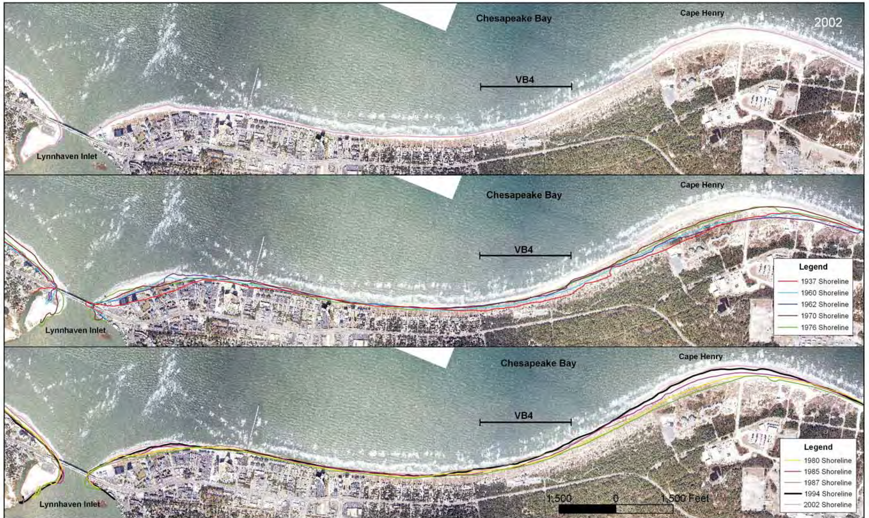
Figure 11-2-4. High-level orthorectified aerial photography of First Landing State Park and VB4 taken in 2002 as well as all the digitized shorelines.
