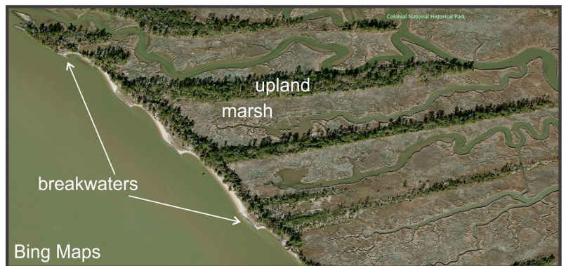
Figure 3-8. Bing map showing headland breakwaters that were built along Jamestown Island's James River shore.
