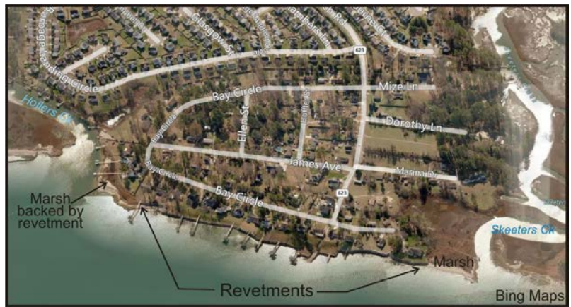
Figure 2-3. Developed shoreline between Hoflers Creek and Skeeters Creek. The shoreline is protected by rock revetments in front of the houses.
