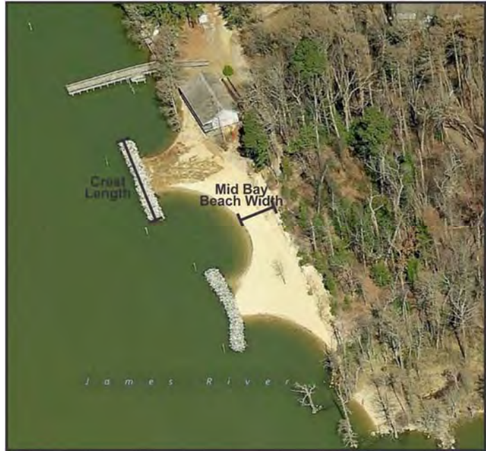
Figure 3-7. Breakwaters along the James River designed to provide a recreational beach as well as storm erosion protection.
