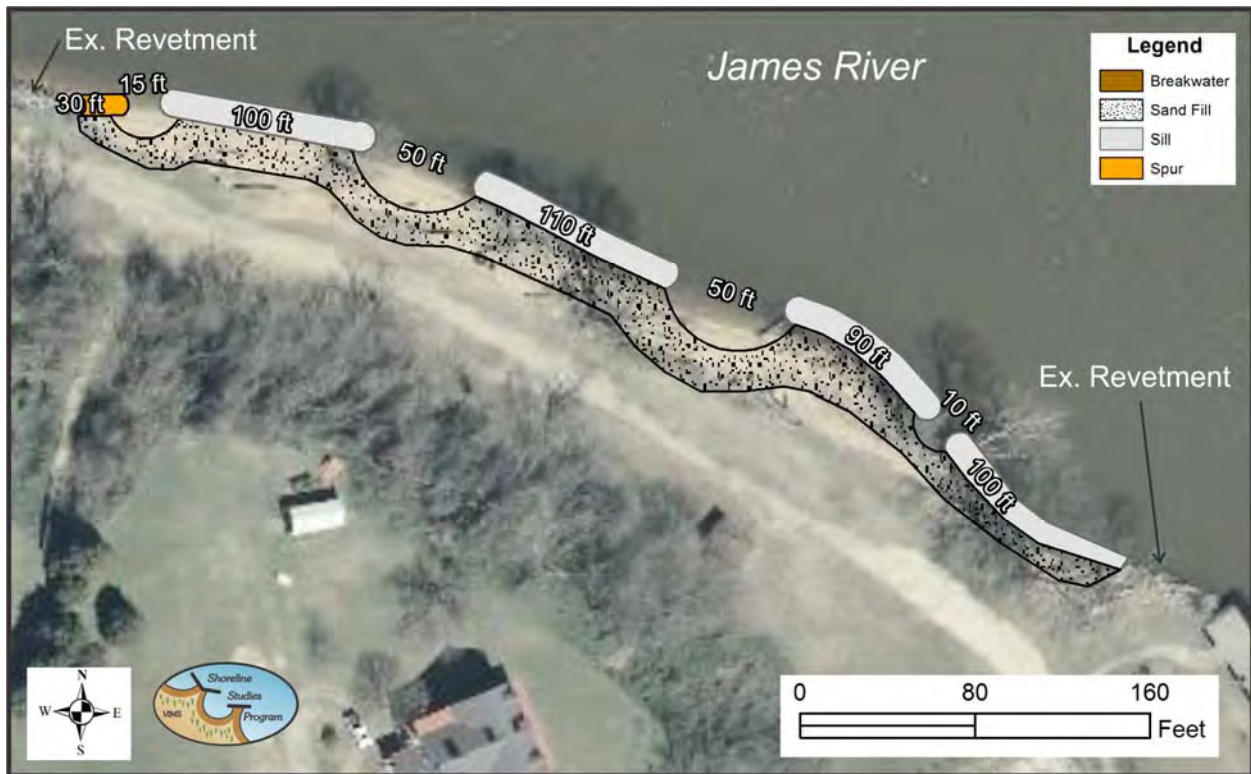
Figure 5-5. Conceptual design of a shore protection system for the eroding shoreline along the park at City Point.
