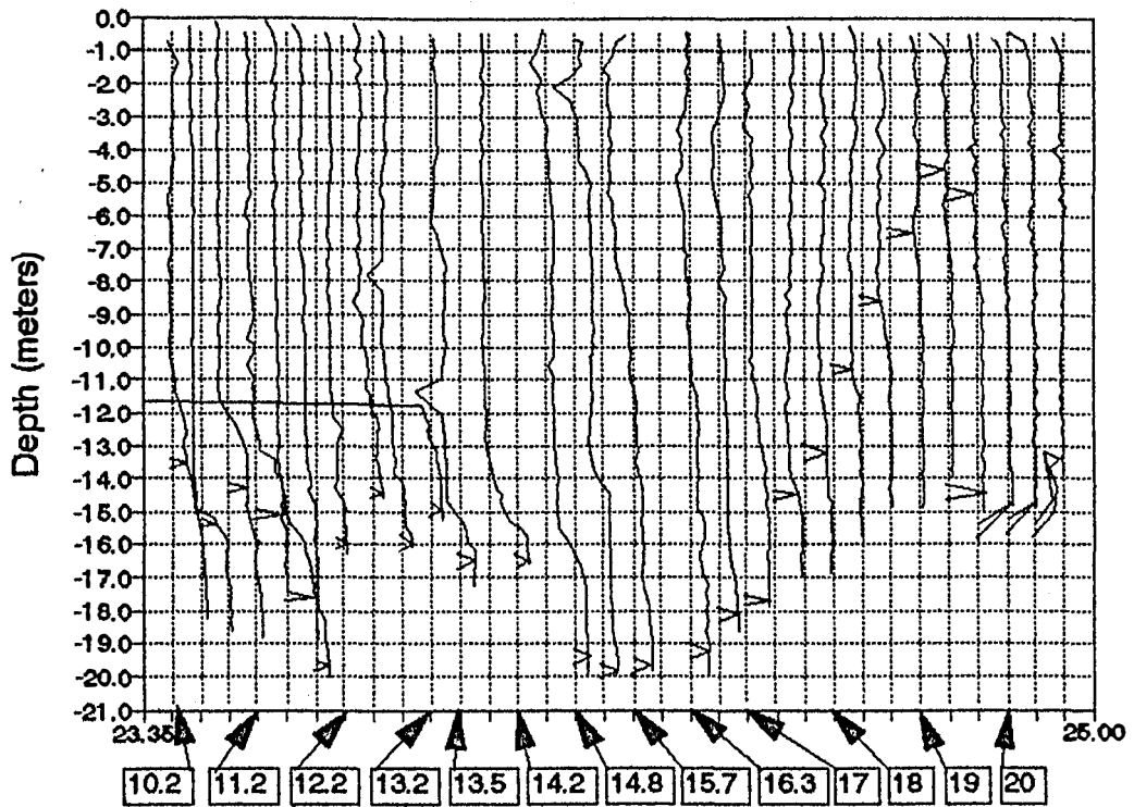
IV-4-8 Sequential plots of salinity with depth along drogue trajectory with offset of 0.05 psu. Vertical lines indicate salinity of 23.40 psu.
