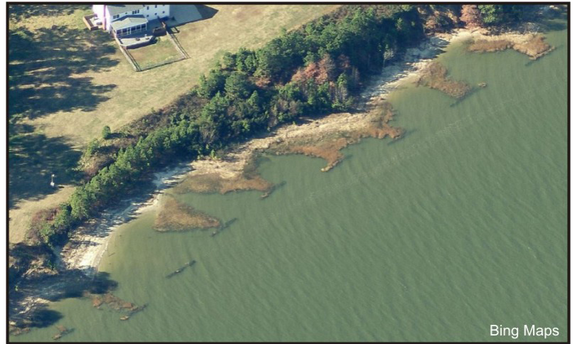
Figure 2-3. Eroding banks, marsh fringe, and shore protection structures along the York River between Queens Creek and Skimino Creek. Several of the structures have been effective maintaining a marsh behind it thereby reducing direct wave impact to the upland bank and slowing erosion.
