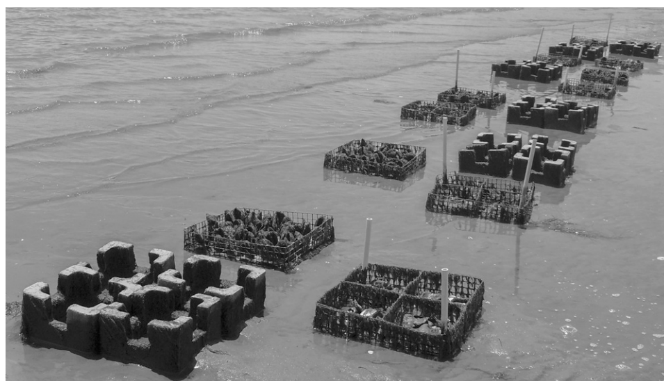
Figure 1. Photograph of the layout of experimental reef substrates used in the field experiments during the conditioning period, including Oyster Castle, unconsolidated oyster shell, and vertically embedded oyster shell in concrete.
