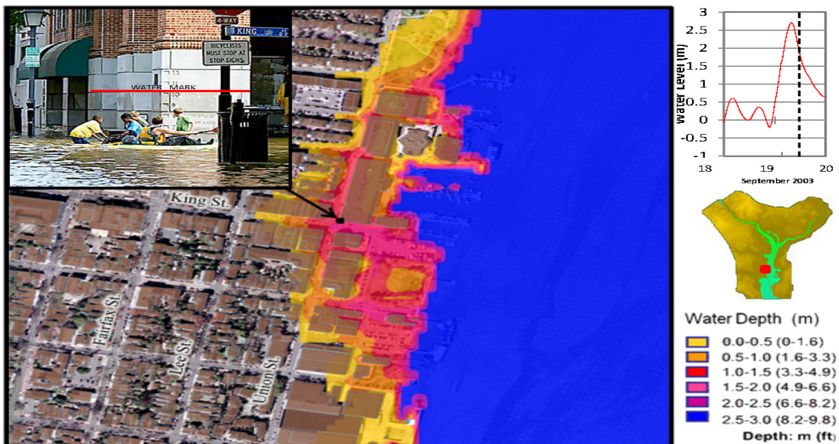
Figure 7. The modeled 2003 Hurricane Isabel-induced inundation in the City of Alexandria, VA. The photograph depicts a high water mark at the intersection of King Street and Union Street showing that the floodwater reached 10.2 feet, approximately 5.5 feet (1.7 m) above the ground level, which is consistent with the modeled inundation at the location, which is between 4.9 and 6.6 feet (1.5–2.0 m).
