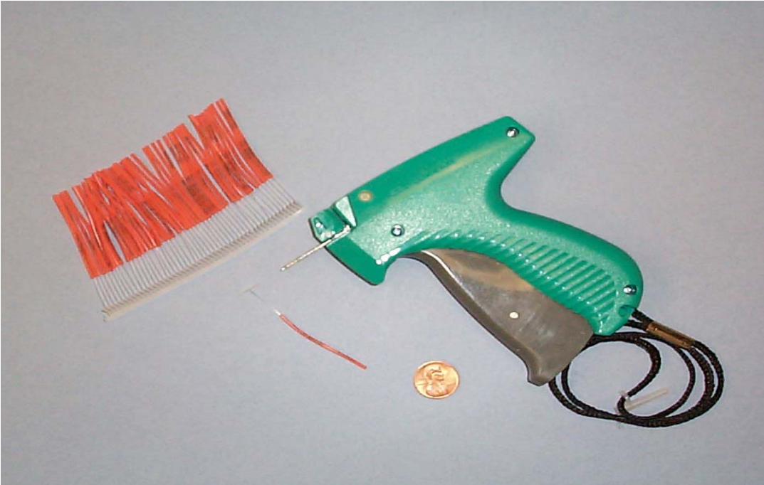
Figure 1. Tagging gun and T-Bar tags and Stainless steel dart tag and applicator (Note: coin for scale – 0.75 inches diameter)
