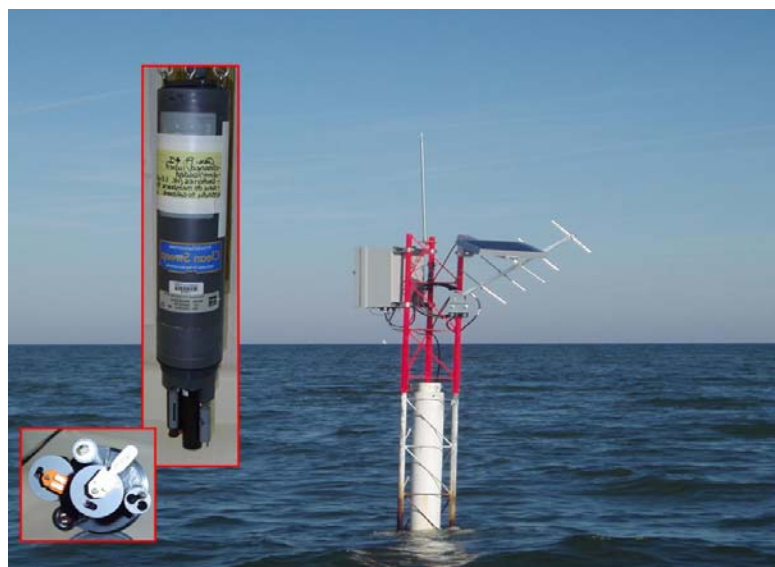
Figure 7.2. Goodwin Island SWMP continuous water quality monitoring station equipped with GOES satellite transmitter. Insert: YSI EDS water quality datalogger. Photo credit: William Reay.
