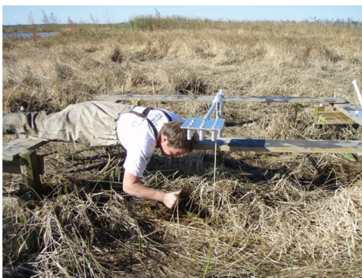
Figure 10.2. Deploying SET to measure sediment accretion on marsh surface. Photo credit: James Goins.
