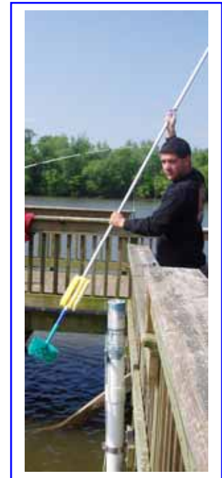
Figure 7.7 Cleaning inside the guard-pipe
