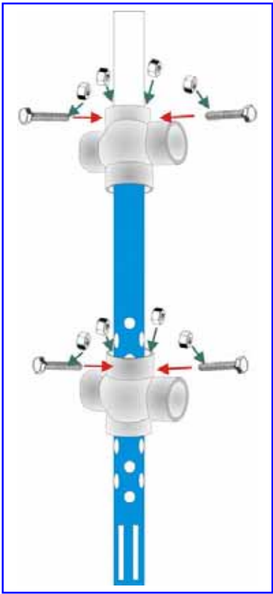
Figure 5.17 Sketch of a guard-pipe fastened to double tees using a bolt and double-nut holding system
