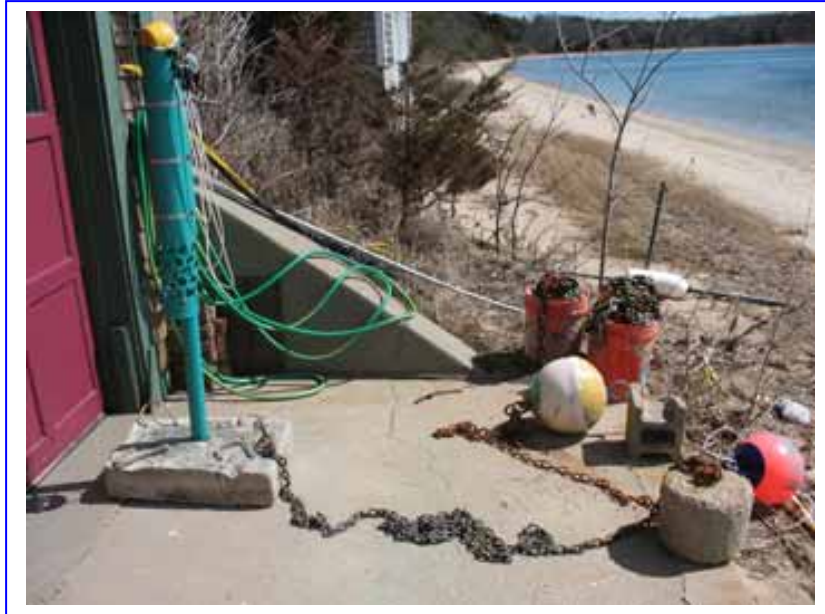
Figure 5.22 View of the station marker buoy attached to a round cement weight
