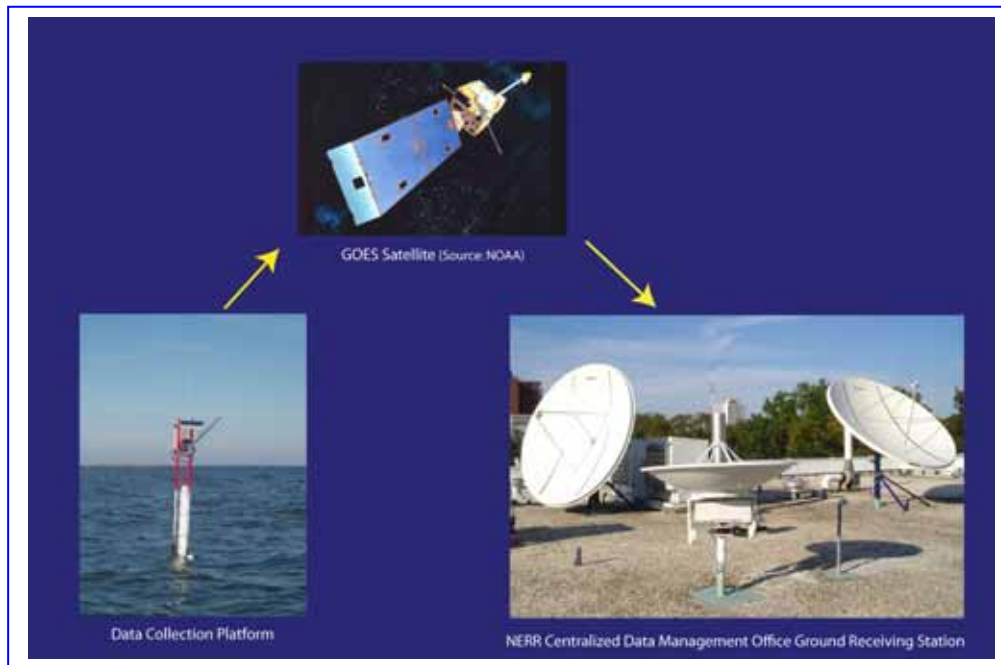
Figure 6.2 Major components of NERR's telemetry system
