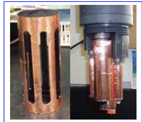
Figure 7.1 Copper tape on guard and probes
