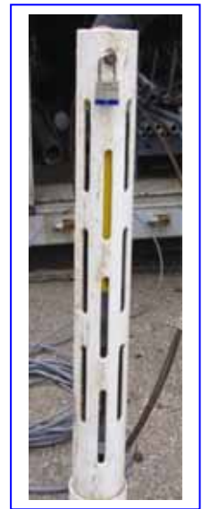
Figure 3.5 Guard-pipe by The Province of British Columbia
