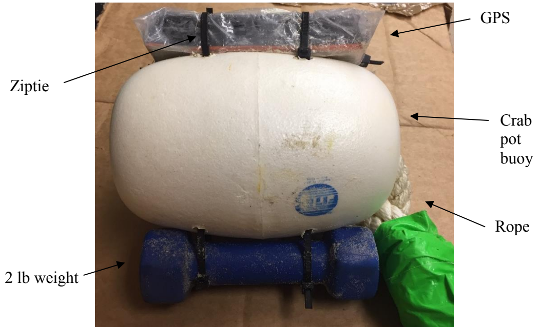
FIGURE A3. Self-righting buoy attachment with GPS for wood-Styrofoam and turtle carcass drifters.
