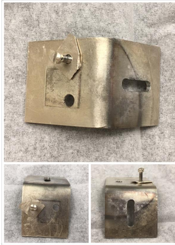
Figure 5.2 Illustration of the OAD setup, including the top view (top), the substrate position (bottom left) and the slot (bottom right).
