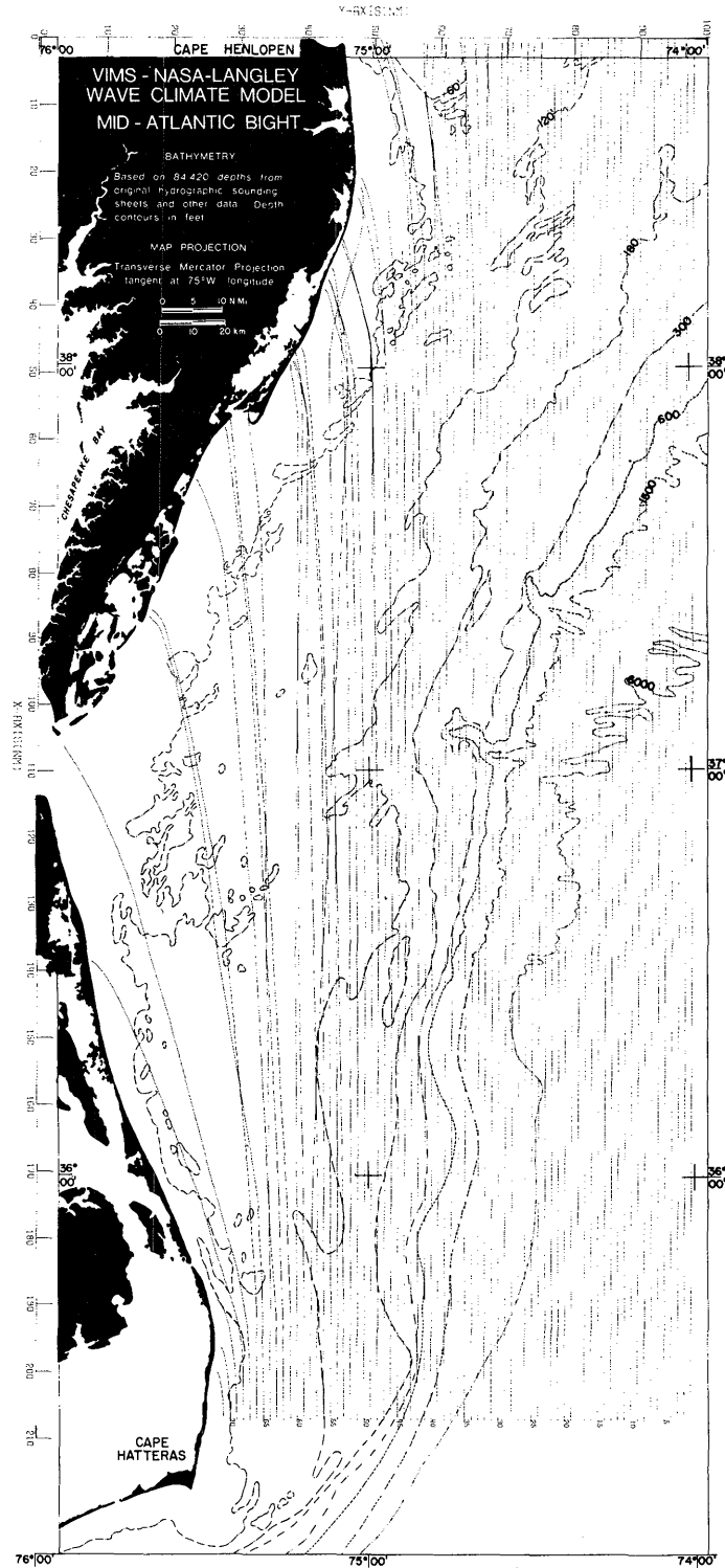
Figure B48.- Wave rays computed with following input conditions: AZ = 180°; T = 6 sec; Tide = 0.
