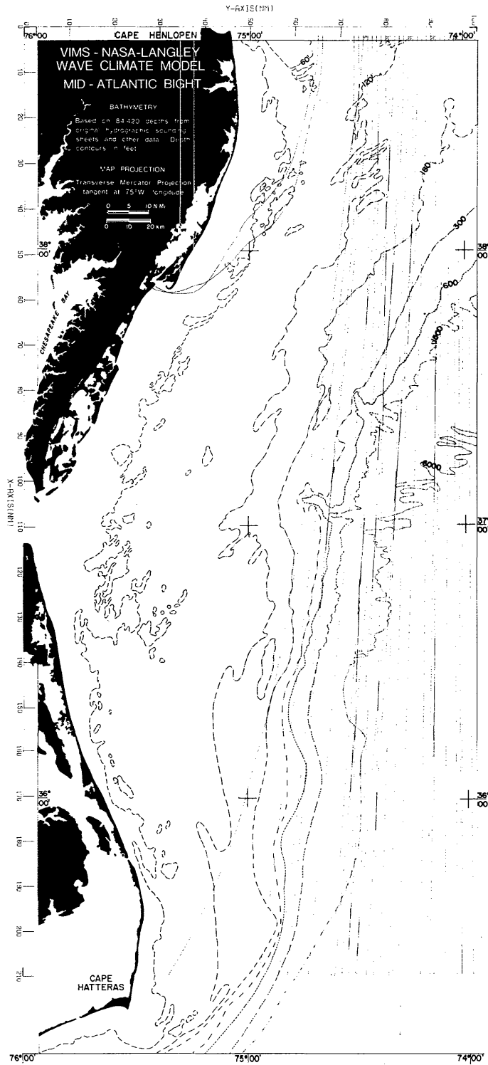
Figure B3.- Wave rays computed with following input conditions: AZ = 0°; T = 8 sec; Tide = 0.
