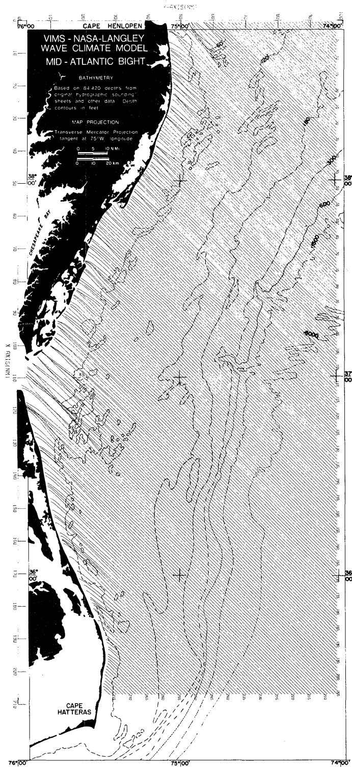
Figure B36.- Wave rays computed with following input conditions: AZ = 135°; T = 6 sec; Tide = 0.
