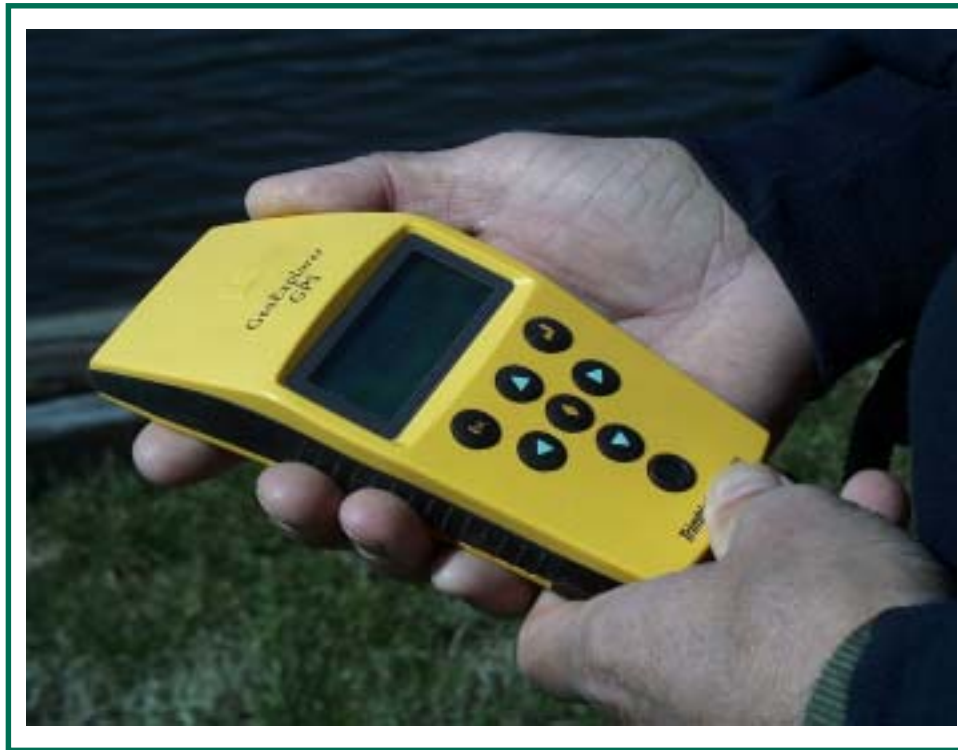
A hand-held Trimble Geo-Explorer logs field data observed from the boat.
