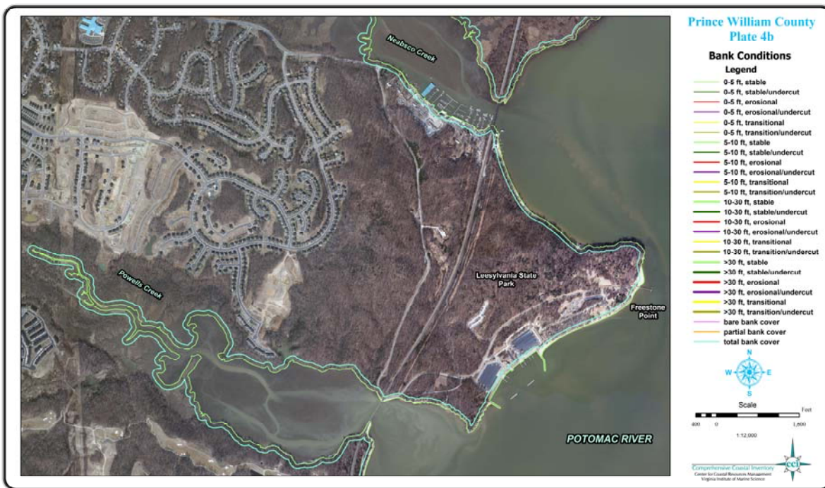
Figure 7. Map illustrating bank conditions for plate 4 in the County of Prince William
