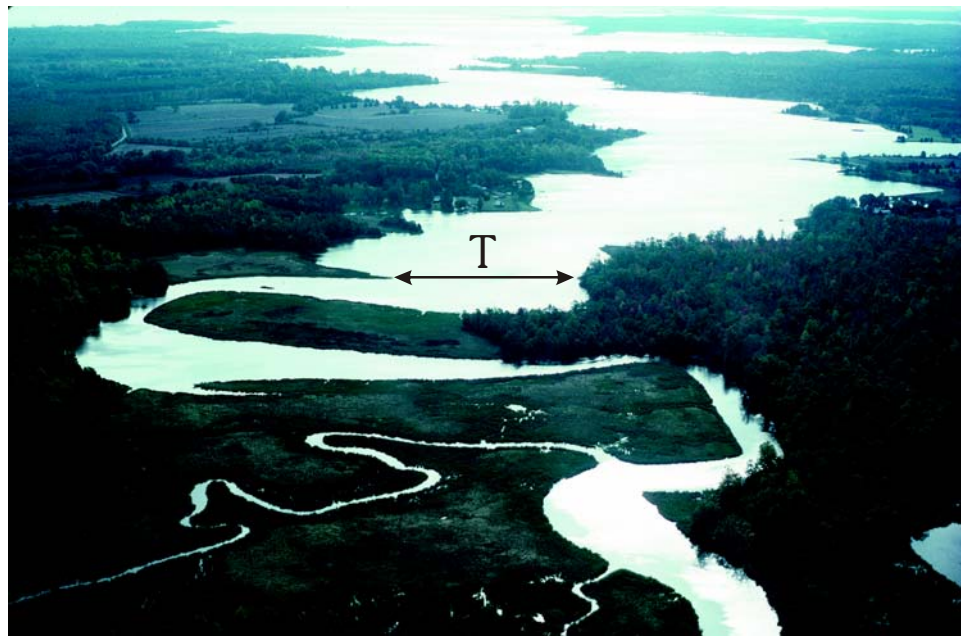
Figure 2 Broad marshes in foreground give way to fringing marshes downstream where there is greater fetch exposure. At the transition point (T), shoreline processes go from tidally dominated to wave dominated (Ware River, Va).
