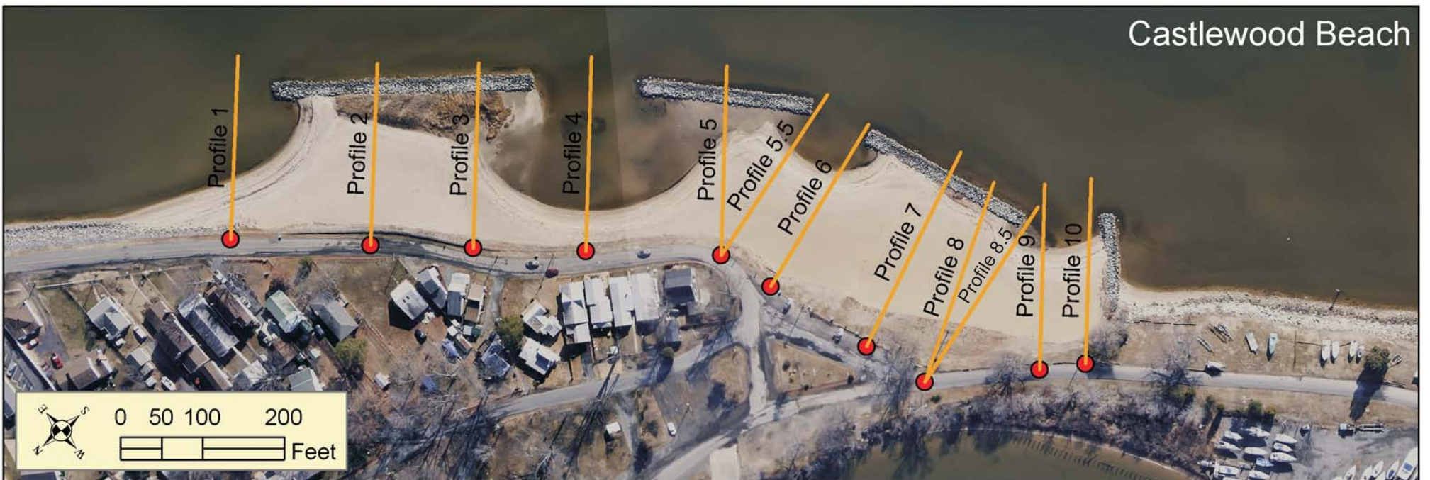
Figure 2. Profile baselines for Central Beach and Castlewood Beach in the Town of Colonial Beach. Also shown are the Volume Calculation Cells (VCC) for Central Beach.
