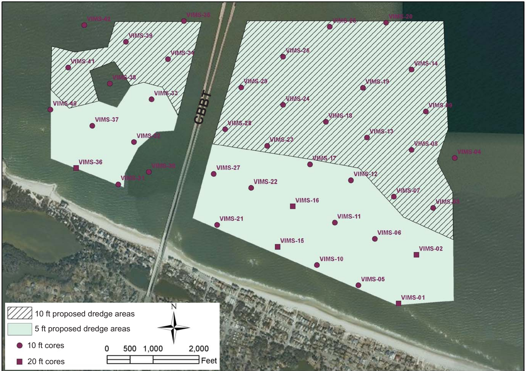
Figure 3-3. Proposed dredge scenarios for the areas on the east and west side of the Chesapeake Bay Bridge Tunnel. 2009 VGIN image.
