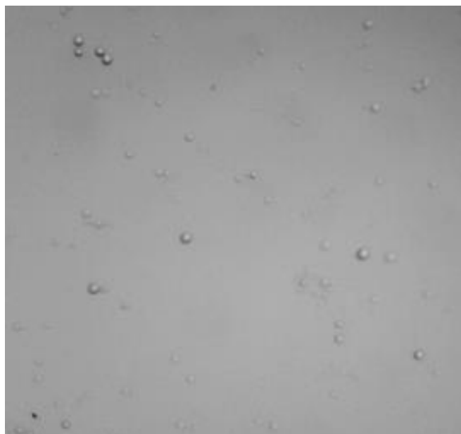
Figure 2. Average diameter of a MNB size is 7 \mu\text{m}
