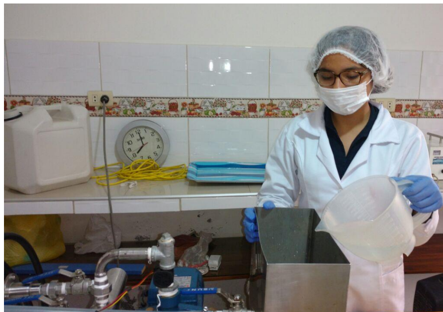
Figure 2. Entering wastewater to the nanobubble generator
