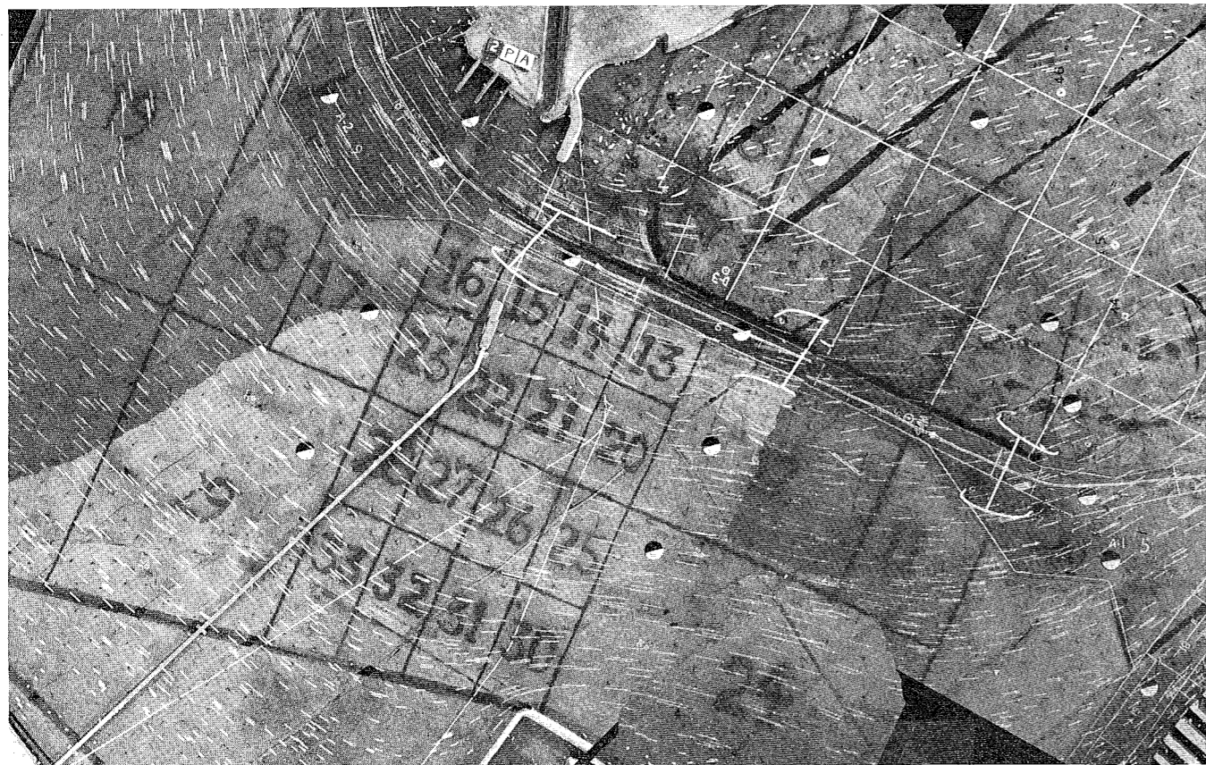
Figure 2 – Second Hour of Tidal Cycle, Typical Confetti Time-Lapse Photograph of Configuration 1A
