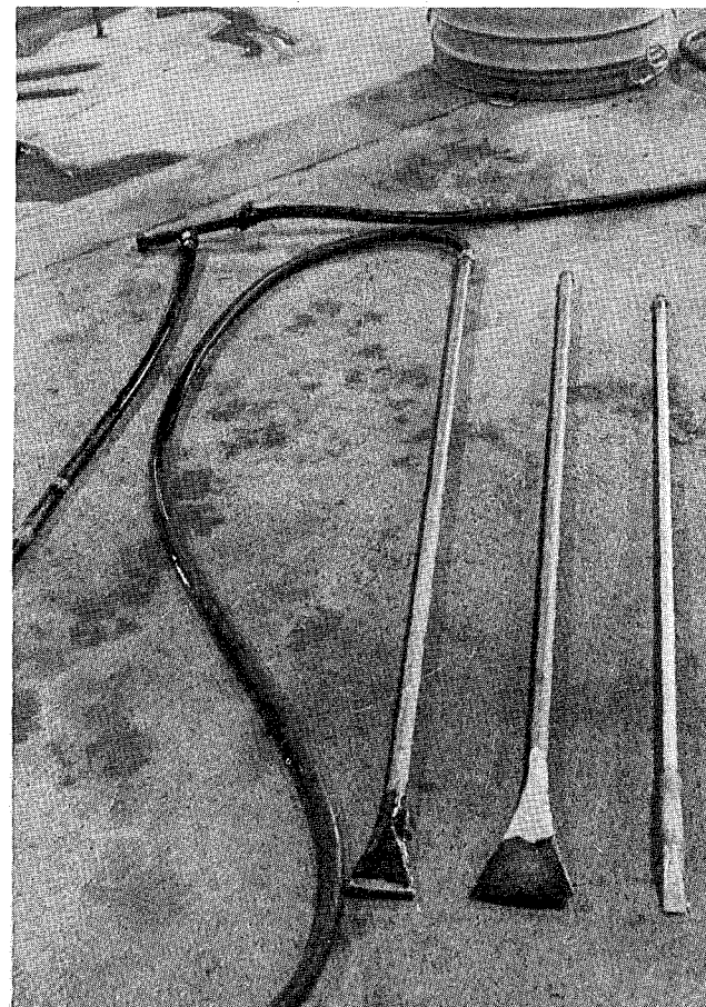
Figure 11 – Hydraulic-Model Aspirator Used by Waterways Experiment Station, showing additional nozzles of varying size.
