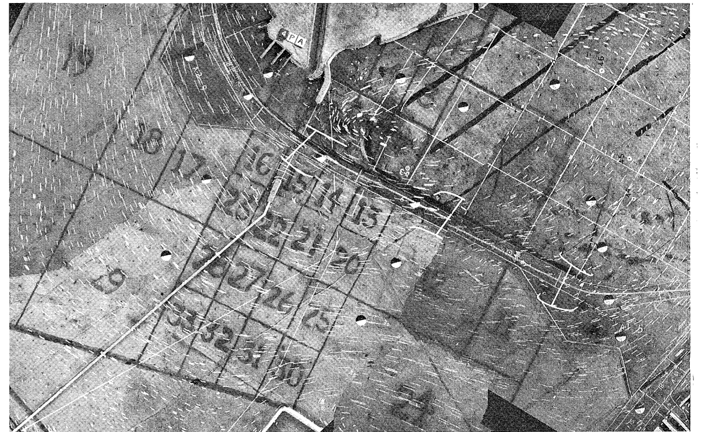
Figure 3 – Fourth Hour of Tidal Cycle, Typical Confetti Time-Lapse Photograph of Configuration 1A
