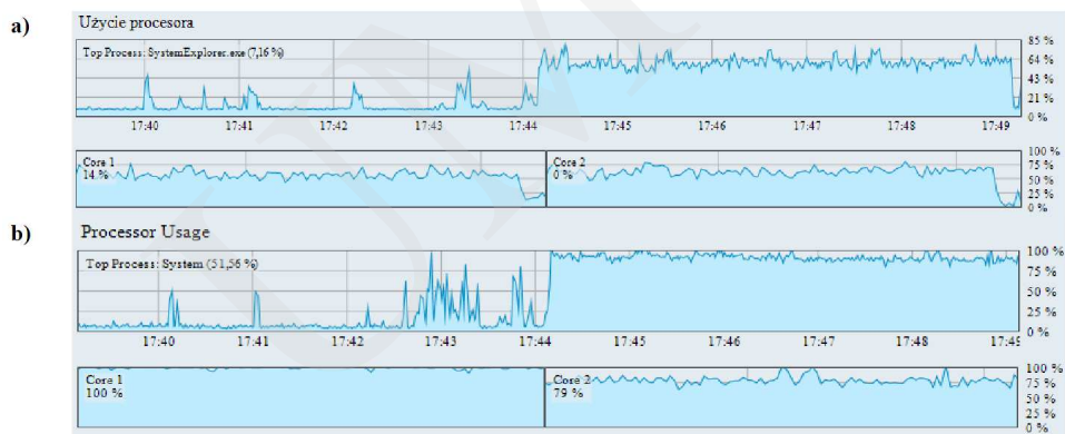
Fig. 10. The CPU usage for the VPN tunnel with L2TP/IPsec in FastEthernet: a) server; b) client.
