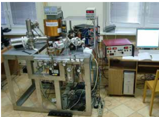
Figure 1: Overall view on the 60° magnetic sector mass spectrometer. The inlet system is installed at the front of this picture. The ion source is on the right side and the collector assembly on the left. The mass spectra and isotope analyses are computer controlled.
