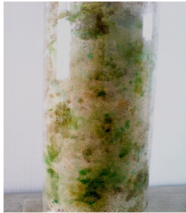
Fig. 3. Algal and fungal growths in the sandy soil taken as an example seven months after wetting-and-drying cycles
