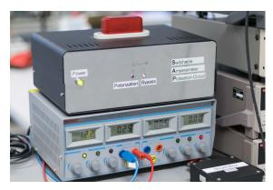
(f) Switchable Amperemeter Protection Circuit (SAP) box.
