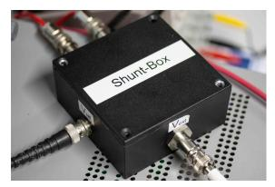
(b) Close up of the "Shunt Box", which forms the central hub of the hysteresis measurement setup and contains all necessary circuitry and connectors to attach the other components as well as the exchangeable reference resistor  $R_{\rm ref}$ .
