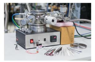
(b) Vacuum measurement chamber standing on the hot plate.
