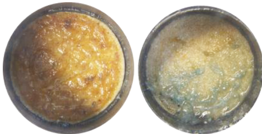
Figure 7-24: Gelled material at front and back face of filtration core #3
