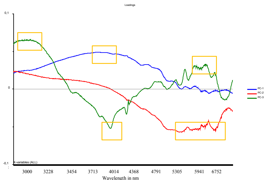
Figure 15: The loading plot of the first 3 PC's of the MWIR data
