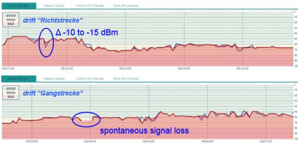
Figure 3: Fluctuation in signal strength at the site “Wlhm-Std.-S
