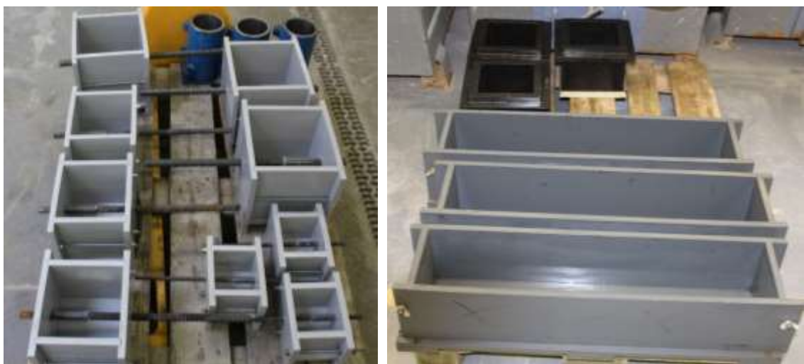
Figure 4.6 Formwork ready before concrete placement
