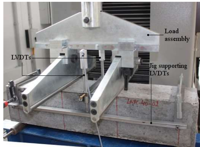
Figure 4.9 Flexure test setup
