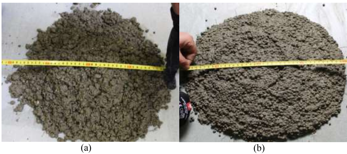
Figure 4.5 Measurement of slump flow (a) NWFC (b) LWFC
