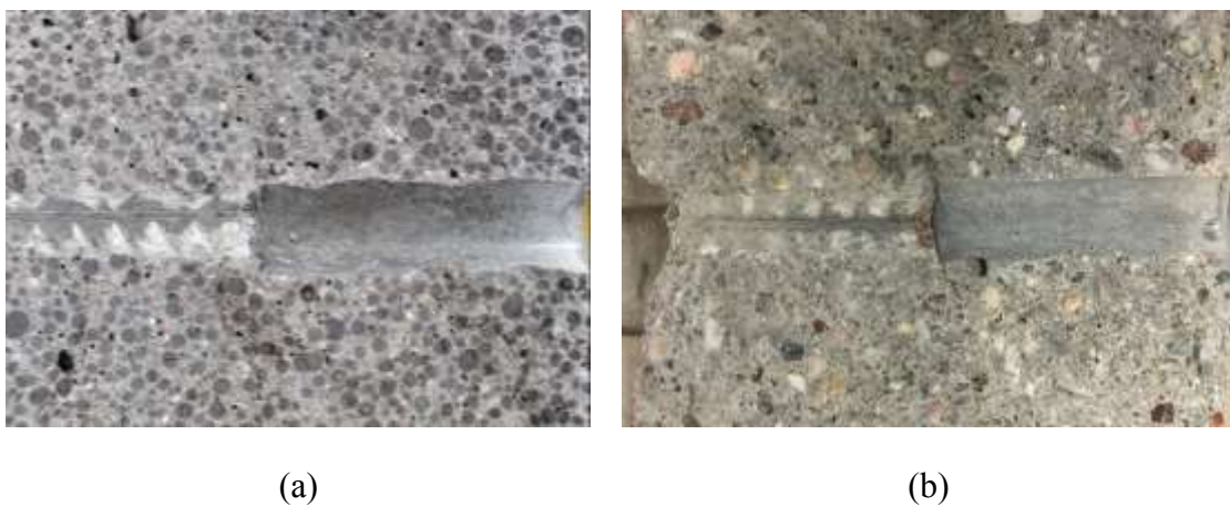
Figure 6.5 Overview of specimens after bond test (a) LWC, (b) NWC
