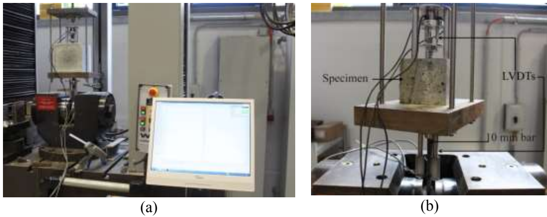
Figure 4.15 (a) Pull-out test setup (b) close-up of specimen
