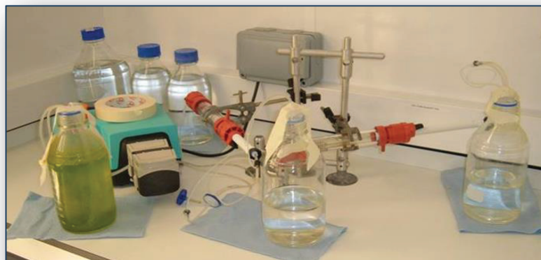
Fig. 3: Flow through culturing system setup permitting continuous supply of fresh medium, here the supernatant from a natural complex phytoplankton assemblage. The supernatant is supplied at a low flow rate via a peristaltic pump to the suspension of millions of agarose droplets within the bioreactors (XK16/20 chromatography column, Pharmacia).
