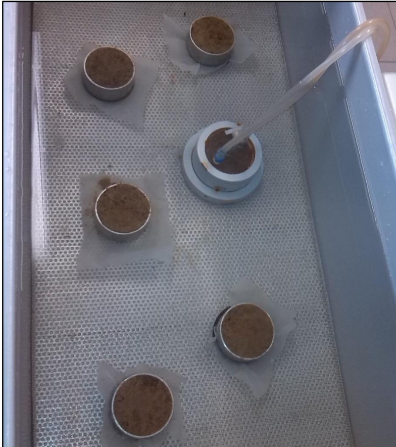
Figure 17. Soil samples are in the Hauben permeameter
