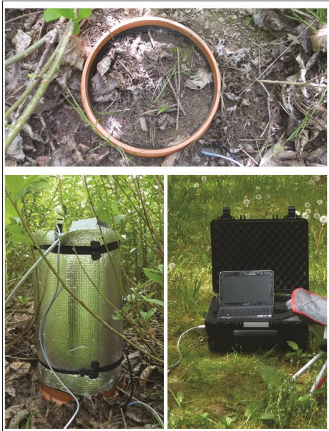
Figure 9. Manual soil respiration measuring system (SEMACH-FG). Top: PVC collar; Lower-left: gas collection chamber; Lower-right: registration and steering unit.
