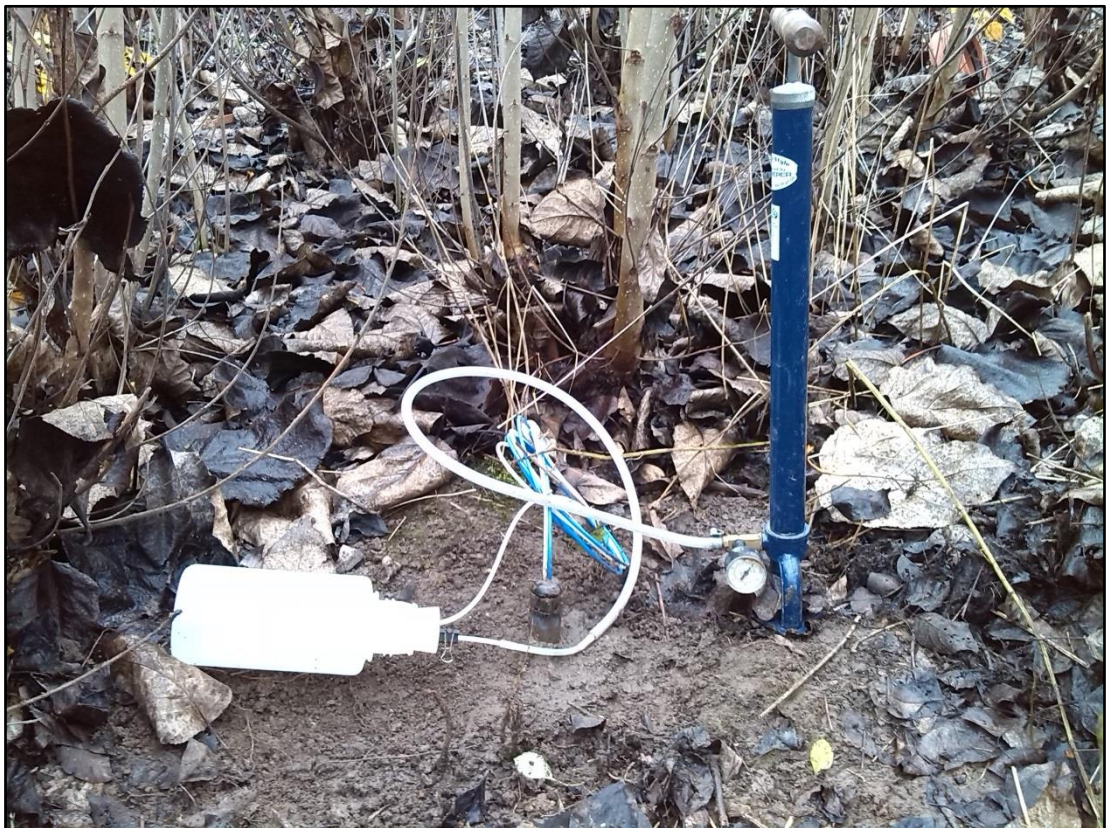
Figure 14. Pressure vacuum soil water sampler at the SRF site with a hand-vacuum pump
