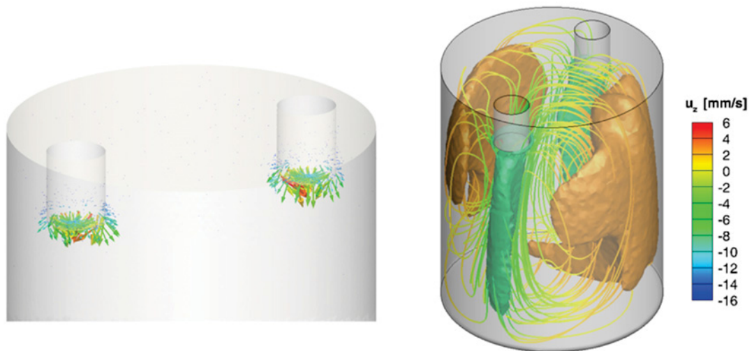
Figure 3.12: Numerical simulations for the situation of an applied direct current at I_{DC}=48A : (a) structure of the electromagnetic force, (b) three-dimensional flow structure.
