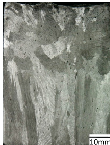
Figure 3.1: Solidified macrostructure of Al-7wt%Si alloy on the longitudinal section of the solidified samples without electric currents.
