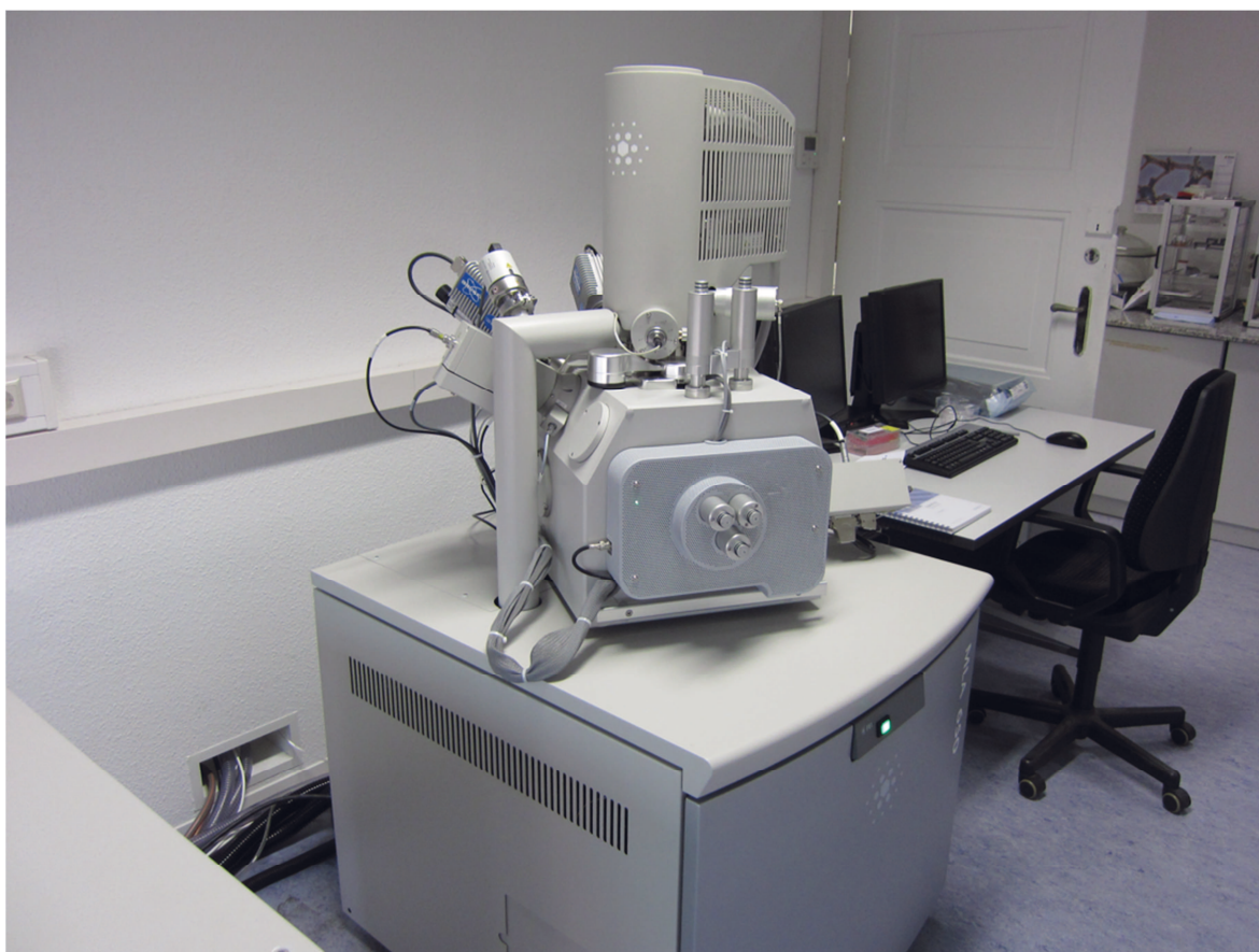
Fig. 16: MLA 650 FEG system in the Geometallurgy Laboratory at the Department of Mineralogy, TU Bergakademie Freiberg.
