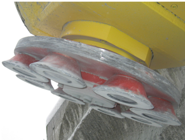
Fig. 10. A view of the wear of the plate with disc tools (Gospodarczyk et. al 2010)
