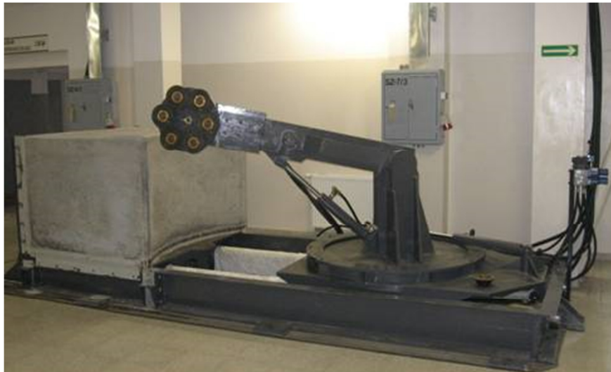
Fig. 4. A view of a lab stand for testing mining process of hard rocks with disc tools (Gospodarczyk et. al 2011), (Kotwica et. al 2013)
