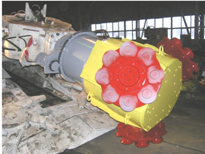
Fig. 7. A view of a head with asymmetrical disc tools of complex motion trajectory on the arm of the KR 150 roadheader, ready for field tests (Gospodarczyk et. al 2010)
