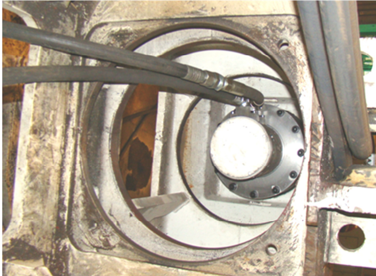
Fig. 9. A view of mounting the hydraulic engine to drive plates with disc tools in the arm of the KR 150 roadheader (Gospodarczyk et. al 2010)
