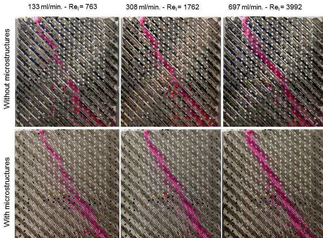
Figure E.1 Wetting behaviour for water in two different corrugated sheets with and without microstructures. Top – Mellapak 350Y without microstructures ; Bottom – Mellapak 350Y B with microstructures.
