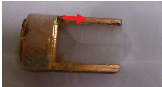
Figure 6-14 Pure chitosan freeze-casted with copper inlays on both sides of the mold (configuration b). Red arrow = freezing direction.
