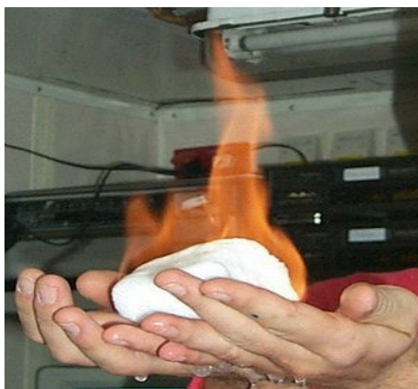
Figure 7: Gas Hydrates; “Burning Ice Effect” [after Gary Klinkhammer [15]]
