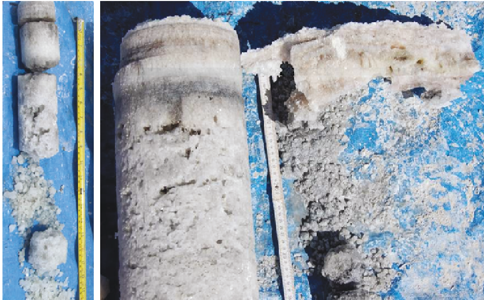
Figure 37: 3-inch (left) and 8-inch (middle) salt core samples from 0 – 1 m depth of the salt crust at drilling site 08-CEN. The upper approx. 20 cm are very hard and dense without high, visible porosity. Below that part there is a friable zone with very high porosity of approx. 30-40%. Right: Cross-section of the remained crust of a brine pool formed within the friable horizon of the near-surface part of the salt crust.
