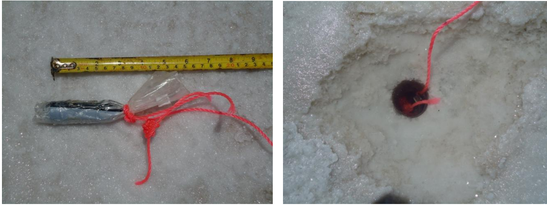
Figure 16: Installation of the Cera-Divers in shallow depth in the Uyuni salt crust.
