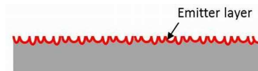
Figure 40 Schematic illustration of a mc-Si wafer after emitter diffusion.
