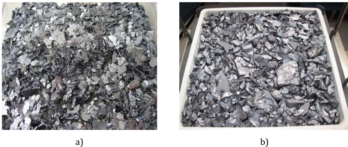
Figure 31 Image a) shows the 4N+Al “flake like” feedstock. Image b) depicts a quartz crucible coated with silicon nitride and filled in with silicon feedstock chunks.
