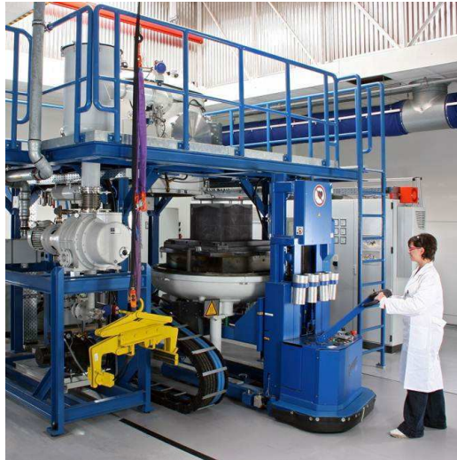
Figure 32 Crystallization furnace in SIMTEC laboratory at Fraunhofer ISE.
