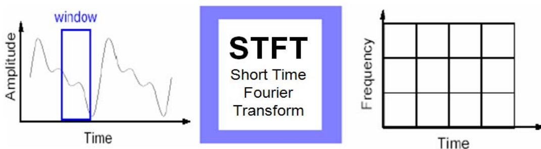
Fig. 2.12: Theory of the short time Fourier transformation (redrawn) (Guan et al., 2004)
