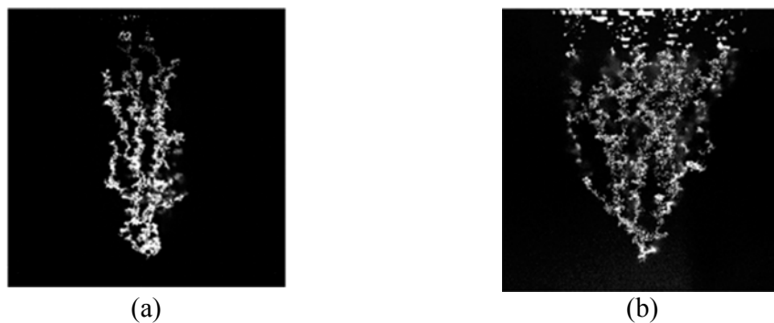
Fig. 4.2: Steady-state channelized flow pattern in: (a) 0.5 mm-GBS, and (b) 1mm-GBS, for Q_g = 10 ml/min (Krauss, 2007).
