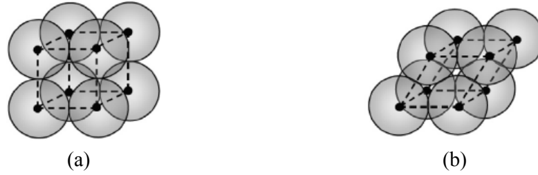
Fig. 2.11: Visualization of: (a) simple cubic packing, and (b) cubic-face-centered packing (Geistlinger et al., 2006).
