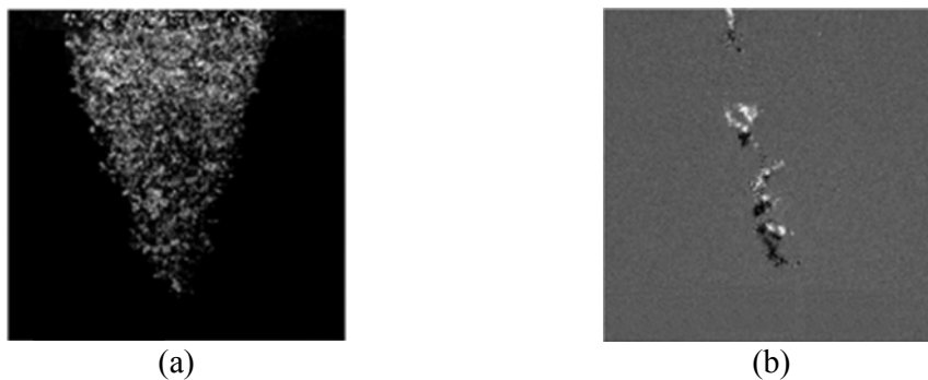
Fig. 4.3: Gas flow pattern in 2 mm-GBS: (a) at quasi steady-state, (b) for difference of two subsequent images ( \Delta t = 1 sec) in quasi steady-state (Krauss, 2007).
