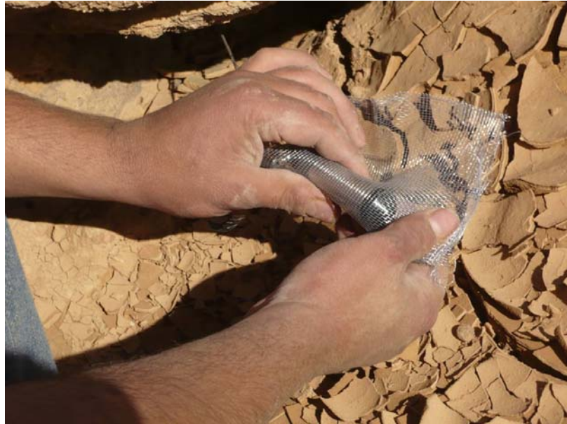
Figure 10. Diver installation in the study area to measure streamflow magnitudes
