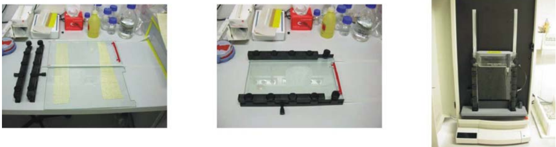
Figure 5-2: Gel-apparatus for genotyping on the automated LI-COR Sequencer (Model 4200 - 11G). Two 41 cm long glass plates, separated by 0.2 mm spacer were overlaid and clamped into two appropriate rails. Finally this cassette was inserted into the sequencer.
