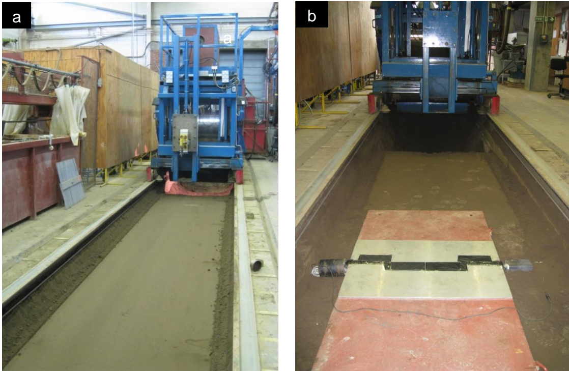
484 Fig. 3. Soil bin laboratory (a: soil surface preparation, b: pressure mapping system 485 placed on the steel plates)
