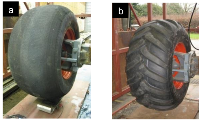
Fig. 4. Smooth (a) and treaded (b) Trelleborg T421 Twin Implement 600/55-26.5 tyres
