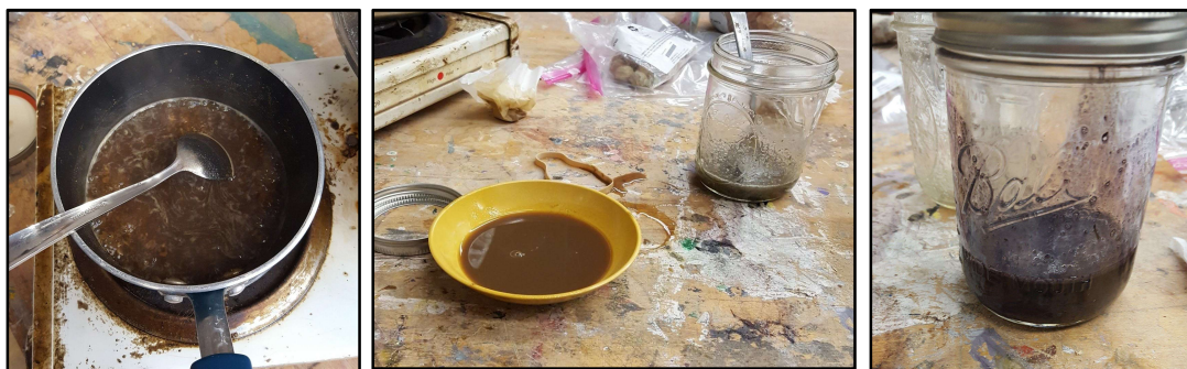
Fig. 3. Left to right: oak galls and water after two hours of boiling; filtered oak gall mixture (yellow bowl) and remade gum arabic/iron (II) sulfate mixture (glass jar with spoon); ink immediately after mixing all ingredients together.
