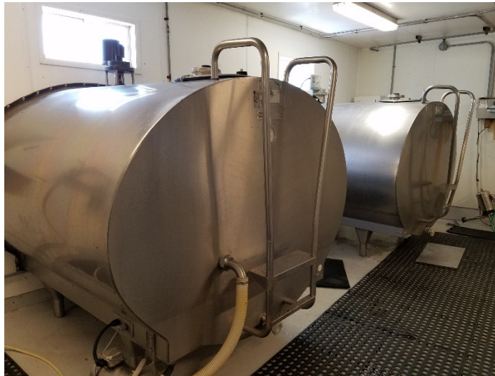
Figure 14: Bulk tanks for milk at WCROC. The bulk tanks store milk after it is extracted from the cow. The bulk tanks include circulation technology that stirs the milk, and uses a scroll compressor to keep the milk cool until it is picked up by the purchaser.
