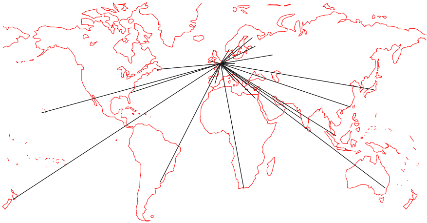
Figure 10.3: A globally distributed GP system (Langdon, 2005a). The server is the centre of the star architecture, with the lines connecting it to users around the world. The users evolved snowflake patterns using a continuously evolving L-System, and their (subjective) preferences provided the fitness measure used to drive the system.
