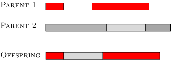
Figure 7.3: Typical linear GP crossover. Two instructions are randomly chosen in each parent (top two genomes) as cut points. The code fragment excised from the first parent is then replaced with the code fragment excised from the second to generate the child (lower chromosome).
